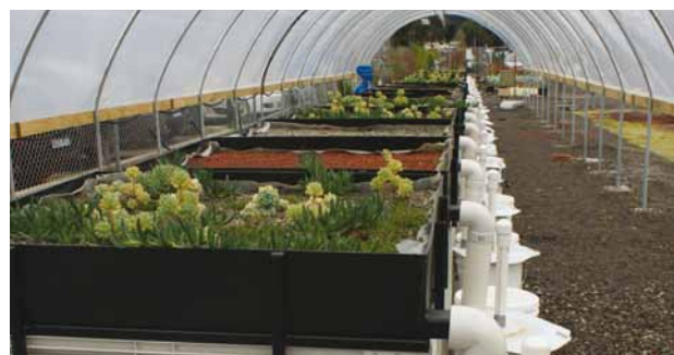
Green roofs research at The University of Melbourne includes survival experiments in greenhouses and on roofs, and hydrology experiments in controlled environments under cover
